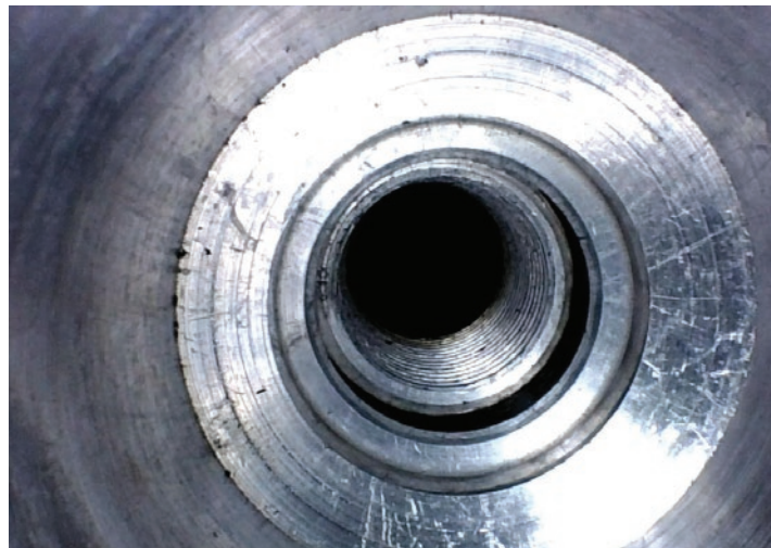
Photo above: Spark plug port inspection
